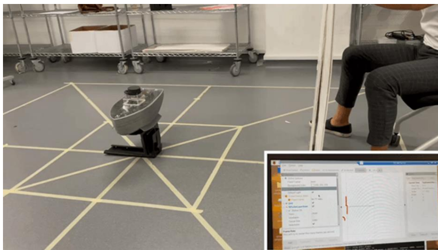
Figure 45: Testing of the Lidar from a distance of 100cm
