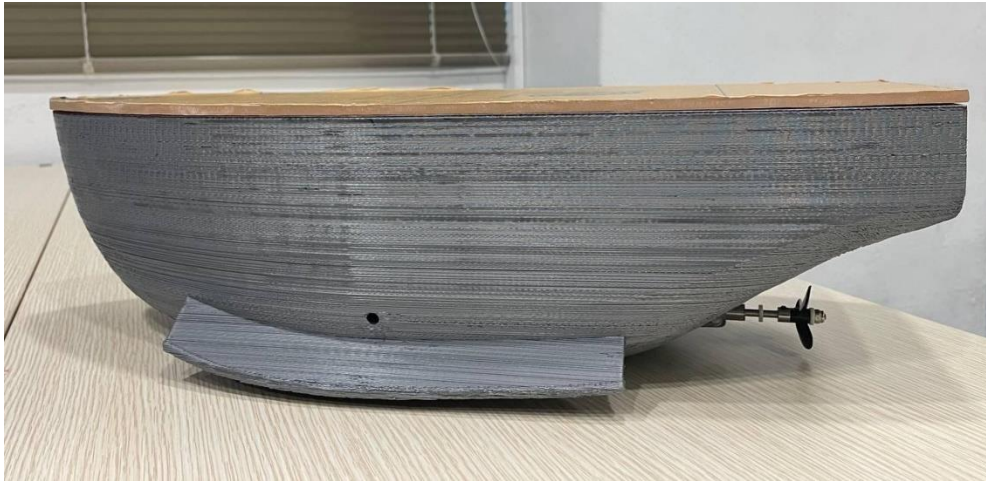
Figure 31: Housing Deck attached to the Hull
